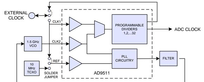
The synthesizer can generate any frequency from 45 to 128 MHz and most frequencies from 128 to 150 MHz. See the specification section for the range of un-settable frequencies.
